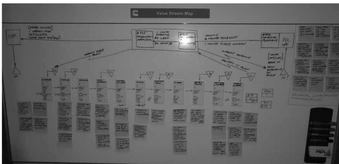
Figure 3: Current state VSM - Connecting rod line
